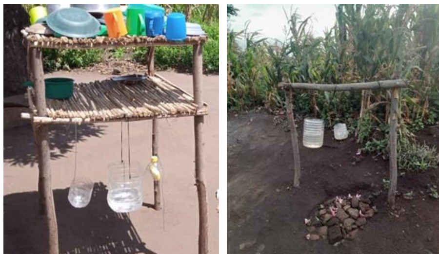
Photo 11. Examples of leaky tins installed attached to a bamboo rack (left), freestanding, 3-pole leaky tin design (right)
